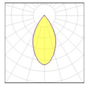
Lamp type Nominal lamp power Total flux Luminous efficacy LED 45 W 3425 lm 76 lm/W CCT CRI LOR Total power
