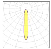
LED Lamp type Nominal lamp power 27 W Total flux 2625 lm Luminous efficacy 97 lm/W
