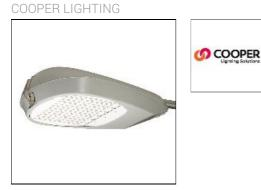
Die-cast aluminum housing and door with stainless steel bail latch, Optical design creates consistent distribution and scalability, Choice of 12 high-efficiency, patented AccuLED Optics<sup>™</sup>, Standard in 4000K (+/- 275K) CCT and nominal 70 CRI, IP66 Rated LightBARs, Suitable for operation in -40°C to 40°C ambient environments, 120-277V 50/60Hz, 347V 60Hz or 480V 60Hz operation, Proprietary circuit module withstands 10kV of transient line surge, Five-year warranty
