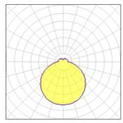
CCT 5000 K Lamp type LED Nominal lamp power 29 W CRI 80 LOR 100% Total flux 2100 lm Luminous efficacy 72 lm/W ULOR 16% Total power 29 W
