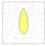
Lamp type LED CCT 3000 K Nominal lamp power 8 W CRI 80 Total flux 550 lm LOR 100% Luminous efficacy 69 lm/W Total power 8 W
