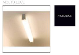
Messina, Wall-/Ceiling Luminaire made of extruded, anodized aluminum; end caps anodized aluminum; Side Cover of white satin acrylic; homogeneous, shadow-free light, Light emission by all sides; high quality Louvre made of coated composite material, glare reduction of 60 °, suitable for computer workstations; IP 20;
