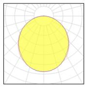
CCT 3000 K Lamp type LED Nominal lamp power 29 W CRI 80 100% Total flux 1600 lm LOR Luminous efficacy 55 lm/W Total power 29 W
