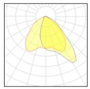
1 x LED Nominal lamp power 72 W LOR 81% Lamp flux 8460 lm Total flux 6860 lm Luminous efficacy 118 lm/W Total power 80 W CCT 3000 K CRI 80
