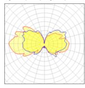
Lamp type Nominal lamp power Total flux Luminous efficacy LED 12.07 W 1068 lm 88 lm/W CCT
