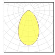
LED CCT 2962 K Lamp type Nominal lamp power 4 W CRI 85 Total flux LOR 100% 219 lm Luminous efficacy 55 lm/W Total power 4 W
