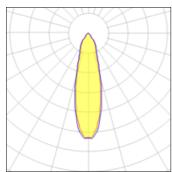
Lamp type CCT 2700 K LED Nominal lamp power 3 W CRI 90 Total flux 191 lm LOR 100% Luminous efficacy 64 lm/W Total power 3 W
