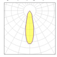
LED CCT 2700 K Lamp type Nominal lamp power 3 W CRI 90 Total flux LOR 100% 191 lm Luminous efficacy 64 lm/W 3 W Total power
