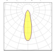
LED CCT 2700 K Lamp type Nominal lamp power CRI 3 W 90 Total flux LOR 100% 191 lm Luminous efficacy 64 lm/W Total power 3 W
