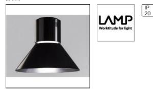
Suspended downlight model STORMBELL 5000 NW FL BK/WH., LAMP brand. Made of shiny black extruded and injected aluminum body with polycarbonate opal ring. Model for COB with neutral white color temperature and control gear included on white decorative rose. Flood aluminum reflector. Insulation class I.
