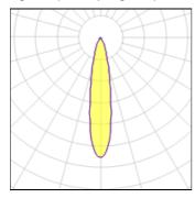
LED CCT 3000 K Lamp type Nominal lamp power 2.75 W CRI 90 Total flux 198 lm LOR 100% 72 lm/W 2.75 W Luminous efficacy Total power
