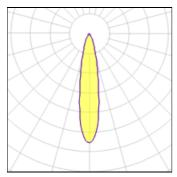
3000 K Lamp type LED CCT Nominal lamp power 2.75 W CRI 90 Total flux 198 lm LOR 100% Luminous efficacy 72 lm/W Total power 2.75 W
