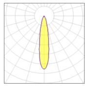
CCT 3000 K Lamp type LED Nominal lamp power 2.75 W CRI 90 Total flux 198 lm LOR 100% Luminous efficacy 72 lm/W Total power 2.75 W
