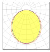
Lamp type Nominal lamp power Total flux Luminous efficacy LED 40.1 W 3608 lm 90 lm/W CCT
