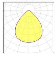
Lamp type LED CCT 4000 K 37.52 W Nominal lamp power CRI 83 Total flux 4050 lm LOR 100% Luminous efficacy 108 lm/W Total power 37.52 W
