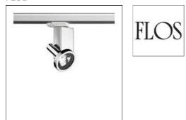
Luminaire for ceiling or three-phase electric track installation. For very low voltage halogen lamps or standard and discharge lamps. Selfextinguishing ceramic or engineering plastic lamp holders, with single-pole, transparent electric wires with double Teflon insulation.
