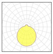
Lamp type LED CCT 3000 K Nominal lamp power 24 W CRI 80 Total flux 2900 lm LOR 100% Luminous efficacy 121 lm/W ULOR 17% Total power 24 W
