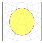
Lamp type LED CCT 3000 K Nominal lamp power 33 W CRI 80 Total flux LOR 100% 2735 lm Luminous efficacy 83 lm/W Total power 33 W
