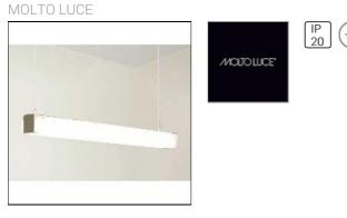
Messina, Hanging lamp made of extruded, anodized aluminum; end caps anodized aluminum; Side Cover of white satin acrylic; homogeneous, shadow-free light, Light emission by all sides; height adjustable without tools, injection transparent, 3x1mm<sup>2</sup>; high quality Louvre made of coated composite material, glare reduction of 60°, suitable for computer workstations; IP 20;
