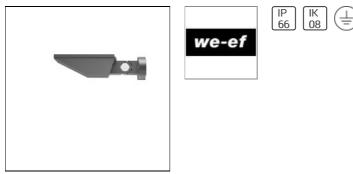
IP66, Class I. IK08. Marine-grade, die-cast aluminium alloy. 5CE superior corrosion protection including PCS hardware. Silicone rubber gaskets. Safety glass, hinged. Integral EC electronic converter. CAD-optimised optics for superior illumination and glare control. OLC® One LED Concept. Factory installed LED circuit board. Luminaire +/-30° tiltable.
