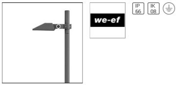
IP66, Class I. IK08. Marine-grade die-cast aluminium alloy. 5CE superior corrosion protection including PCS hardware. Silicone CCG® Controlled Compression Gasket. Safety glass lens, hinged. PMMA OLC® optics for superior illumination and glare control. Recommended mounting height 2.5 - 6.0 m, depending on wattage selected.
