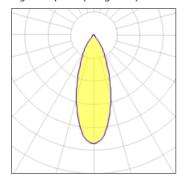
Lamp type LED CCT 3000 K Nominal lamp power 45 W CRI 90 Total flux LOR 100% 3375 lm Luminous efficacy 75 lm/W Total power 45 W
