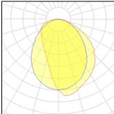
CCT Lamp type LED 3000 K CRI Nominal lamp power 100 W 80 Total flux 13500 lm LOR 100% Luminous efficacy 135 lm/W Total power 100 W
