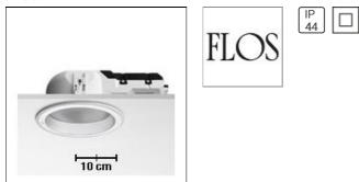
Recessed indoor luminaires for indoor installation for compact fluorescent lamps. Self-extinguishing, thermoplastic white reflector housing; vacuum-aluminium coated anti-glare elements.
