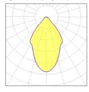
Lamp type LED CCT 3019 K Nominal lamp power 24.4 W CRI 80 Total flux 2062 lm LOR 100% Luminous efficacy 85 lm/W Total power 24.4 W
