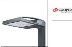
Choice of 16 high-efficiency, patented AccuLED Optics<sup>™</sup>, 3,400 - 61,800 lumens, up to 131 lp/W, Standard in 4000K CCT, 70 CRI, optional 2700K, 3000K, 5000K and 6000K, -40°C to 40°C operating range, 120-277V 50/60Hz, 347V 60Hz or 480V 60Hz operation, IP66 rated housing and LED Light Squares, Thermally conductive polymer heatsink for up to 22% weight reduction, Pole, mast-arm or wall-mounted
