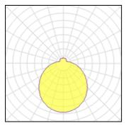
Lamp type LED CCT 4000 K Nominal lamp power 22 W CRI 80 Total flux 2770 lm LOR 100% Luminous efficacy 126 lm/W ULOR 17% Total power 22 W
