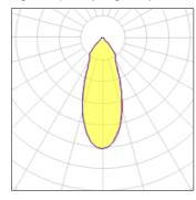
Lamp typeLEDCCTNominal lamp power8 WCRITotal flux617 lmLORLuminous efficacy77 lm/WTotal power
