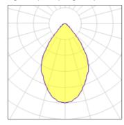
Lamp typeLEDCCTNominal lamp power13.3 WCRITotal flux1076 lmLORLuminous efficacy81 lm/WTotal power
