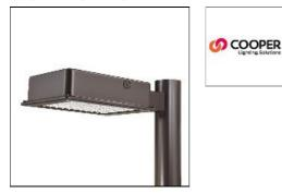
One-piece, die-cast aluminum housing can be pole or wall-mounted, Optical design creates consistent distribution and scalability, Choice of 12 high-efficiency, patented AccuLED Optics<sup>™</sup>, Standard in 4000K (+/- 275K) CCT and nominal 70 CRI, Suitable for operation in -40°C to 40°C ambient environments, 120-277V 50/60Hz, 347V 60Hz or 480V 60Hz operation, Proprietary circuit module withstands 10kV of transient line surge, Optional battery pack and bi-level switching, Five-year warranty
