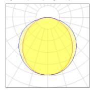
LED CCT 3000 K Lamp type Nominal lamp power 34.6 W CRI 85 Total flux 3470 lm LOR 100% Total power Luminous efficacy 100 lm/W 34.6 W
