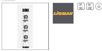
• Lamp LED • CRI Ra > 80 • MacAdam Ellipse 3 SDCM • Colour 3000K and 4000K - Die-cast aluminium housing and extruded aluminium column pre-treated before powder coating ensuring high corrosion resistance - Stainless steel fasteners in grade 316 - Durable silicone rubber gasket -High-efficiency optical reflector or PMMA lens - Clear, acrylic PMMA diffuser - Maximum wind load resistance is 140 km/h - Surge protection 10kV
