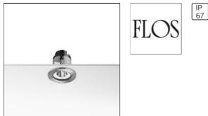
Adjustable recessed luminaire for ceilings or in ground applications, for LEDs or 12 volt halogen QR-CBC 35 lamps. Die-cast aluminum recessed housing, high corrosionresistance. 6mm tempered protection glass. Silicone seals. Stainless steel closing ring with fixing screws. PG9 cable gland with pre-wired 1 metre power loom. Finishes: matt black (04), grey (72), stainless steel (55), stainless steel dark copper (PB), stainless steel gold (PG), stainless steel black (PN).
