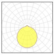
Lamp type LED CCT 4000 K Nominal lamp power 14 W CRI 80 Total flux 1910 lm LOR 100% Luminous efficacy 136 lm/W ULOR 15% Total power 14 W
