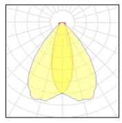
CCT 4000 K Lamp type LED Nominal lamp power 67.3 W CRI 80 Total flux 11548 lm LOR 100% Luminous efficacy 172 lm/W Total power 67.3 W
