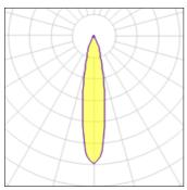
CCT Lamp type LED 4000 K Nominal lamp power 2.75 W CRI 90 Total flux 215 lm LOR 100% Luminous efficacy 78 lm/W Total power 2.75 W
