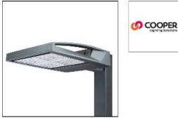
Choice of 16 high-efficiency, patented AccuLED Optics<sup>™</sup>, 3,400 - 61,800 lumens, up to 131 lp/W, Standard in 4000K CCT, 70 CRI, optional 2700K, 3000K, 5000K and 6000K, -40°C to 40°C operating range, 120-277V 50/60Hz, 347V 60Hz or 480V 60Hz operation, IP66 rated housing
