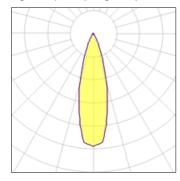
Lamp typeLEDCCTNominal lamp power8 WCRITotal flux556 lmLORLuminous efficacy70 lm/WTotal power
