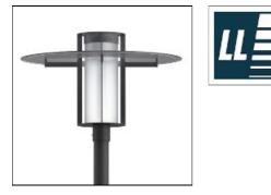
Recommended mounting height 5.00 m max. - Impact-resistant opal polycarbonate cylinder, UV-stabilized - special steel frame, painted -Large aluminium reflector, underside finished in special white paint for max. light reflection - All electrical components on one block - Adapter jack connection - Lamps are easy to change -Available in any RAL or DB color without surcharge - Please order pole dia. 76 mm separately
