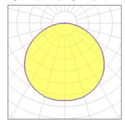
LED CCT 3000 K Lamp type Nominal lamp power CRI 18 W 80 Total flux 1040 lm LOR 100% Luminous efficacy 58 lm/W Total power 18 W
