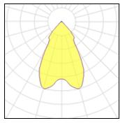
Lamp typeLEDCCTNominal lamp power88 WCRITotal flux9750 lmLORLuminous efficacy111 lm/WTotal power
