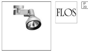
Range of indoor spotlights for accent and general lighting for three-phase track and wall/ceiling installation. Die-cast aluminium alloy, powdercoated optics compartment, diameter 118 mm, composed of an aluminium dissipating element placed above the lamp support, a black thermoplastic screen support ring and 4 mm tempered glass cover. Integrated auxiliary power units for the lamps inside a die-cast aluminium alloy container with powder-coated finish.
