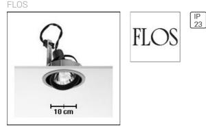
Luminaire for halogen and high-pressure discharge lamps. Injection-moulded aluminium reflector body with powder-coated finish. Lamp support with die-cast aluminium, black powder-coated heat dissipating element. Thermoplastic recessed ring and screening ring, die-cast aluminium, black powder-coated anti-glare ring. 4 mm. tempered glass cover. Stainless steel fixing brackets.
