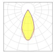
Lamp type Nominal lamp power Total flux Luminous efficacy LED 27 W 1610 lm 60 lm/W CCT CRI LOR Total power 3000 K 80 100%
