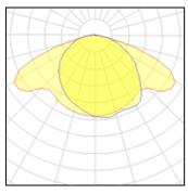
1 x Metal halide lamp Nominal lamp power 70 W LOR 77% Lamp flux 7200 lm Total flux 5556 lm Luminous efficacy 62 lm/W Total power 89 W CCT 3000 K CRI 90
