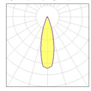
LED CCT 3000 K Lamp type Nominal lamp power 8 W CRI 80 Total flux LOR 100% 503 lm Luminous efficacy 63 lm/W Total power 8 W
