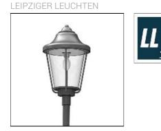
For medium light requirements, mounting heights from 3.00 - 4.00 m. - Luminaire body made of aluminium/galvanized steel sheet - Impactresistant clear polycarbonate attachment, UV-stabilized - Steel tubing galvanized and painted - Adapter jack connection -Available in any RAL or DB -colour without surcharge Voltage: 230V 50Hz Protected to: IP 55 Protection class: I/II Made to DIN VDE 0711 Luminaires generally compensated
