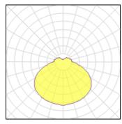
CCT 2700 K Lamp type LED Nominal lamp power 96 W CRI 90 LOR 100% Total flux 2740 lm 29 lm/W Luminous efficacy ULOR 18% Total power 96 W
