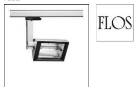
Range of indoor spotlights for accent and general lighting for three-phase track and wall/ceiling installation. Die-cast aluminium alloy, powdercoated optics compartment, diameter 118 mm, composed of an aluminium dissipating element placed above the lamp support, a black thermoplastic screen support ring and 4 mm tempered glass cover. Integrated auxiliary power units for the lamps inside a die-cast aluminium alloy container with powder-coated finish.
