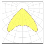
1 x Metal halide lamp Nominal lamp power 400 W LOR 86% Lamp flux 34000 lm Total flux 29310 lm Luminous efficacy 67 lm/W Total power 435 W CCT 5300 K CRI 90
